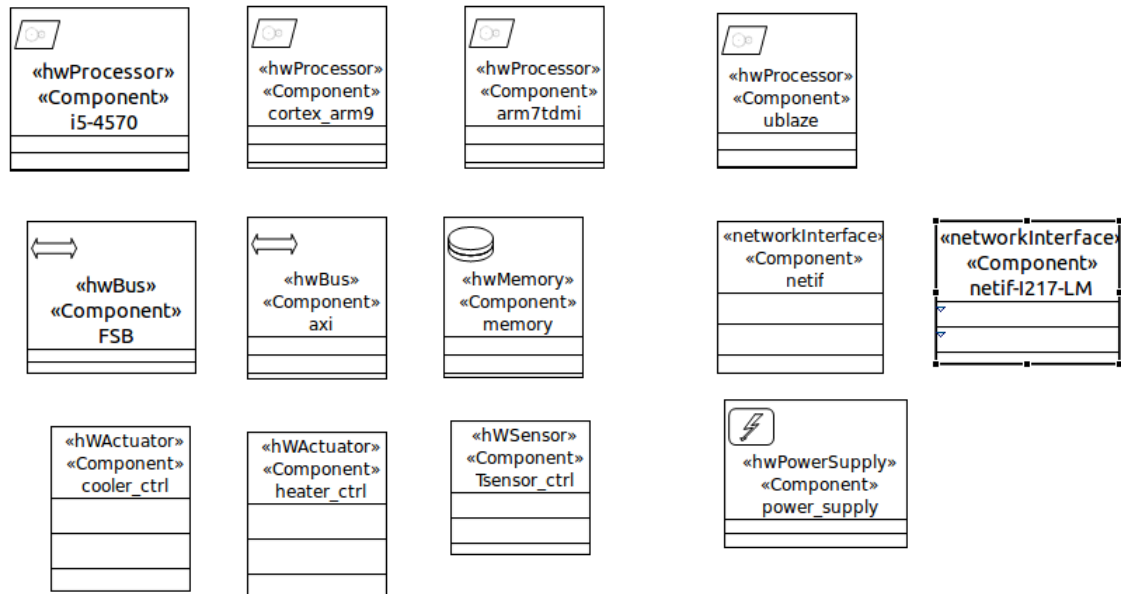
Figure 15. Example of the HW resources view. The set of declared HW components is the union of HW components instanced for each of the internal architectures captured for the three nodes declared in the node view shown in Figure 5.
