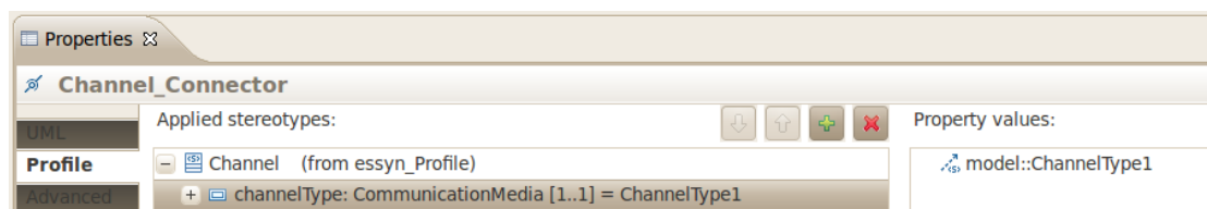
Figure 29 Channel type attached to the Channel connector
