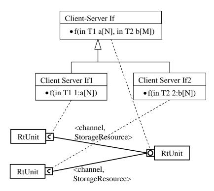
Figure 4 Sketch of a joint-service with data-splitting in the CONTREX UML/MARTE PIM modelling methodology.
